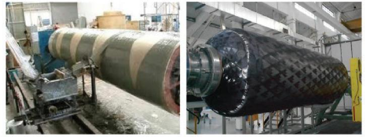
Examples of missile bodies made by filament winding
