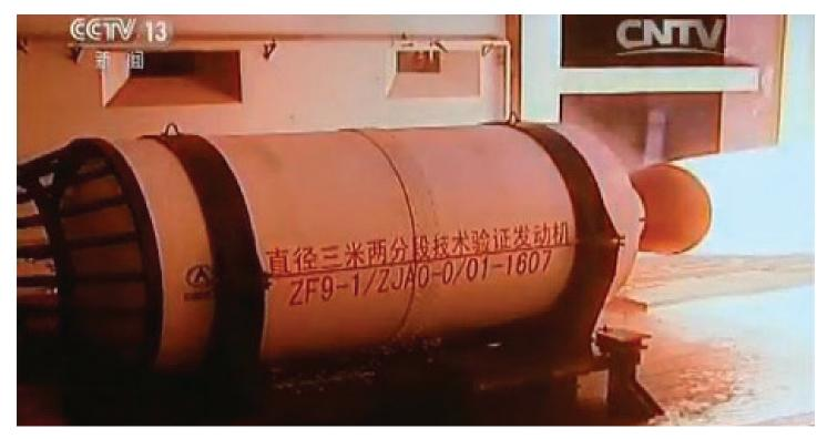
Firing test of 3m-diameter two-stage solid rocket motor in 2016
